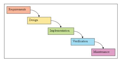
Figure 2. The waterfall process for software development
